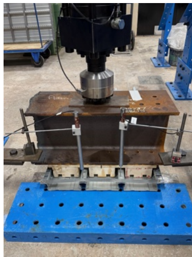
1.50mm End Crush Test
