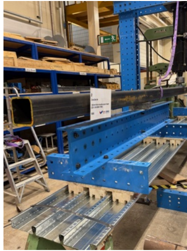
1.00mm Double Span Test
