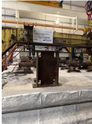
Testing of 1.00mm CompDek 54
