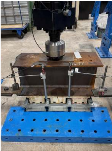
1.50m End Crush Test
