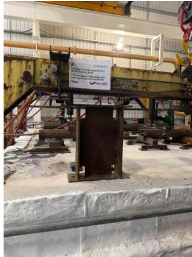
Testing of 1.00mm CompDek 54
