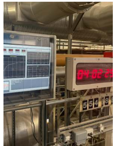
Recording of Fire Test Exceeding 4 Hours Duration
